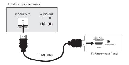
1) Connect the HDMI Cable from the DIGITAL OUT on the back of your DTV or HDMI device, to the DIGITAL-IN on the back of your television.
